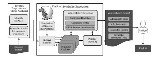
Figure 4.1: Architecture of Teerex [CRD20]
