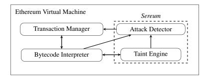
Figure 6.4: Architecture of enhanced EVM with run-time monitoring.
