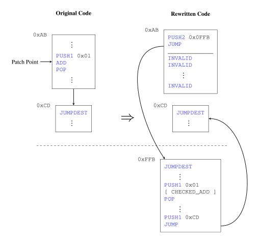
Figure 7.5: Control-flow graph of original and rewritten code. The end of the original contract's code is marked with a dashed line. The original basic block at address OxAB is replaced with trampoline code that jumps to the patched version of the basic block, located at address OxFFB. The patched basic block is appended right after the end of the original contract at address OxFFB. The patched basic block jumps back into the original code at address OxCD.
